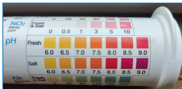
Figure 3. Color range of test strips pads for pH (5n1 test strips).
