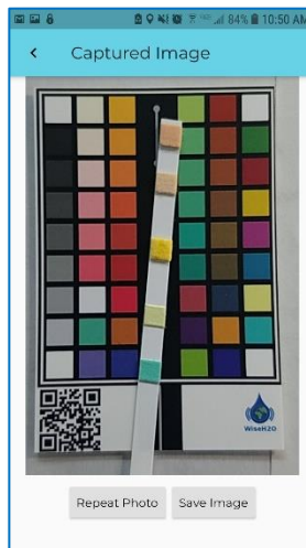
Strip not aligned
